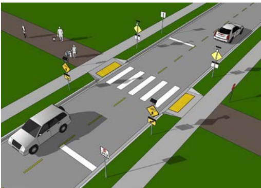
Figure 13. Trail Crossing with Flashing Beacon (RRFB)
