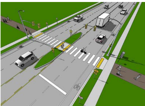
Figure 15. Signalized Trail Crossing with Island
